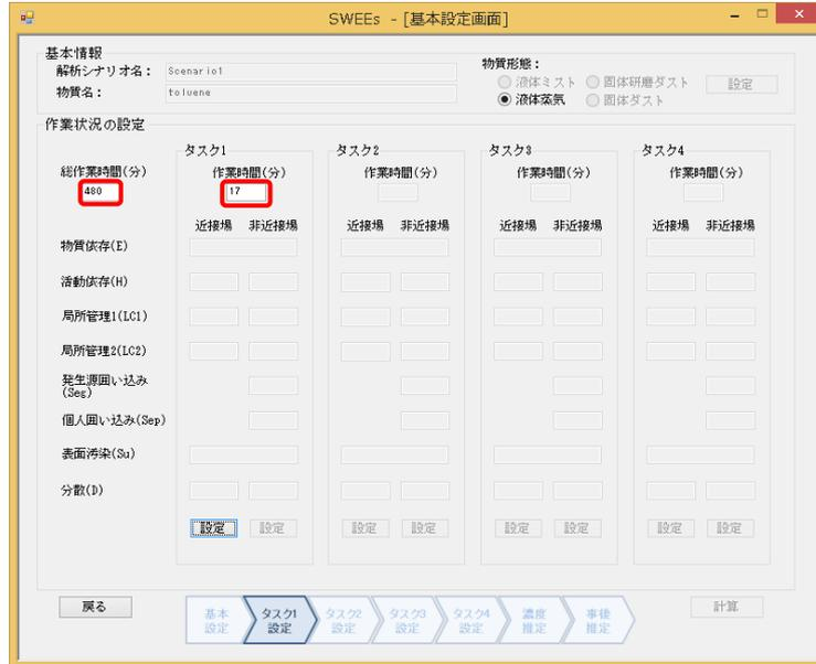
**Figure 5-4 Screen for basic setting: Setting work conditions of task 1**
