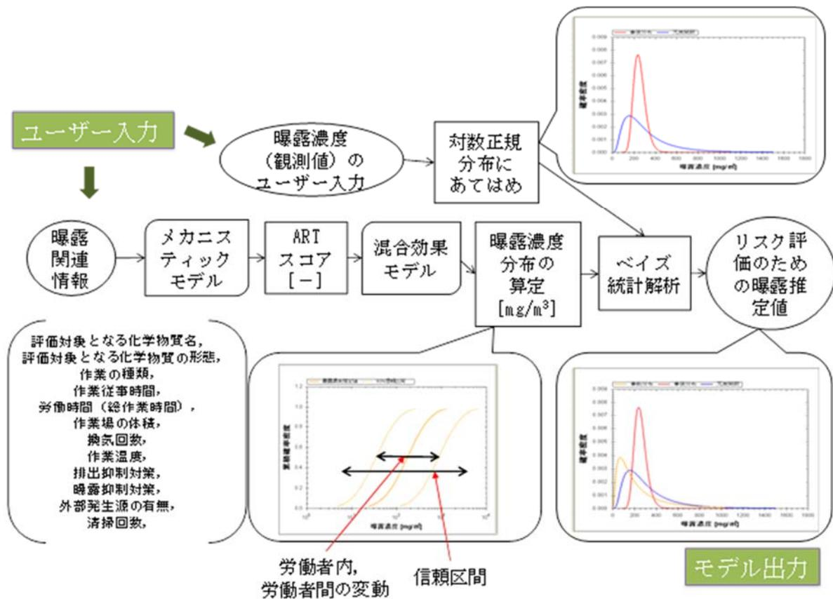
Figure 1-1 Input and output structure of SWEES
