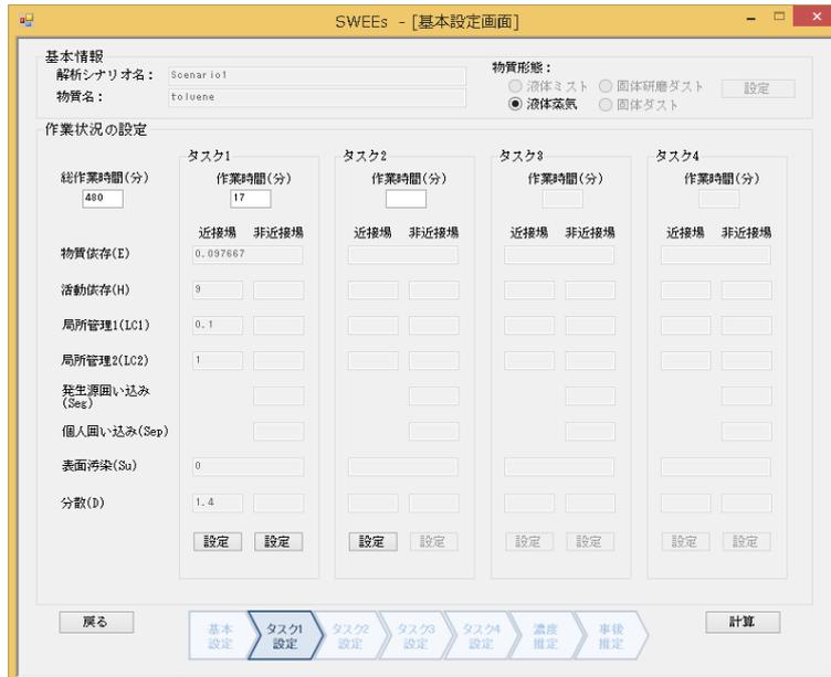
Figure 5-17 Checking the modifying factors on the screen for basic setting (task 1, near field)
