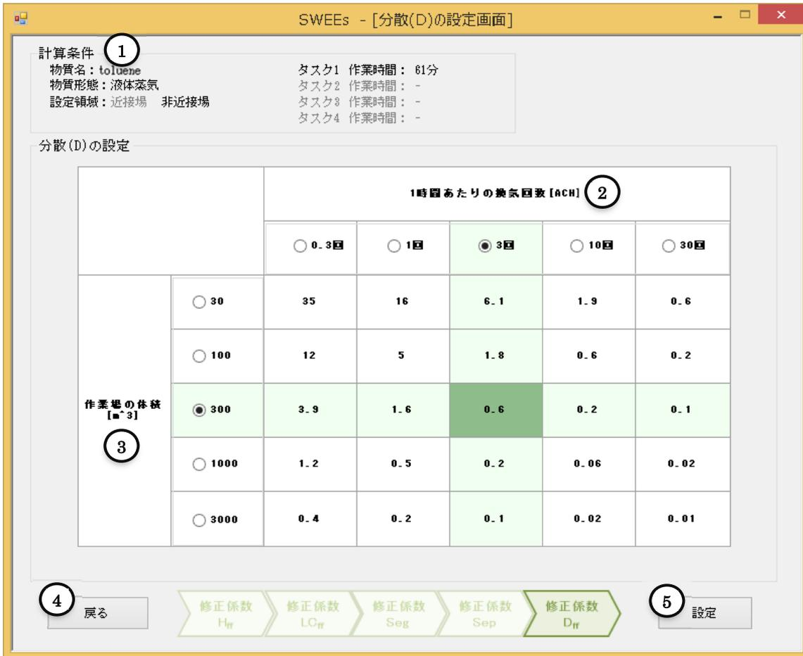
Figure 4-21 Screen for setting the dispersion (D) (If the work duration is more than 60 minutes)
