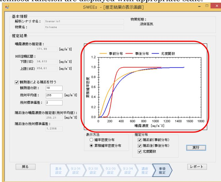
Figure 5-39 Display of superimposed graphs of prior and posterior cumulative probability density distributions and likelihood function
