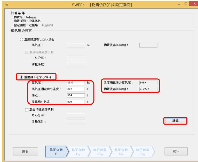
Figure 5-26 Modifying factors: Temperature correction of substance emission potential (E)
