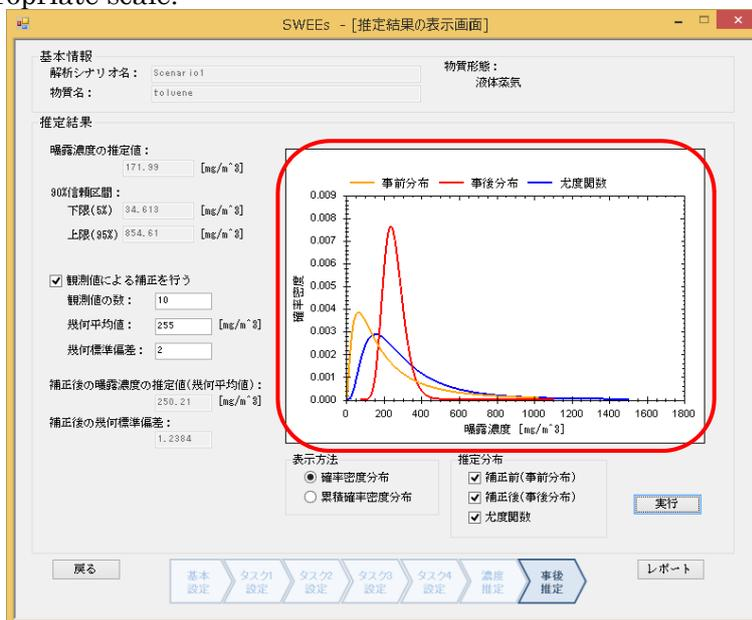
Figure 5-37 Display of superimposed prior and posterior distributions
